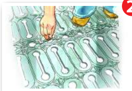
Clip plates together, cut plates with jigsaw if necessary
